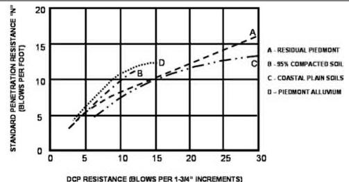
The results of the hand auger boring and DCP tests are summarized on the attached "Hand Auger / DCP Sounding Records." Relative densities and consistencies presented on the logs are inferred from the appropriate correlations in the previous figure.
