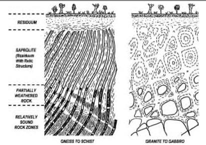
Typical Piedmont Weathering Profiles (After Sowers/Richardson, 1983)
